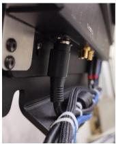
The standard mounting bracket that comes with the vehicle dock features an industry standard VESA 75mm bolt pattern. It must first be removed from the dock by unscrewing the 6x #10-24 screws attaching it to the dock. This allows easy mounting to many preexisting mounts as well as dedicated mounts from Gamber-Johnson.
