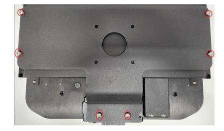
Use the supplied  $4x #\frac{1}{4}-20$  flat head screw and hardware for attaching the back side of the plate to the mount.
